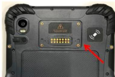
Step 2: Lock 2D module with four screws onto the terminal.
