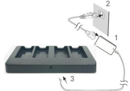
Put the battery into the charger, and the charger will automatically detect the presence of batteries and begin charging.
