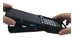
2). Snap in the top two corners of HT730 into the boot case, and make sure HT730 is secured in the boot case.
