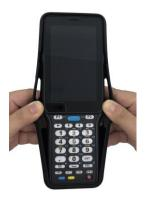
2). Pry the boot case from both edge of the top corner, and take HT730 out.
